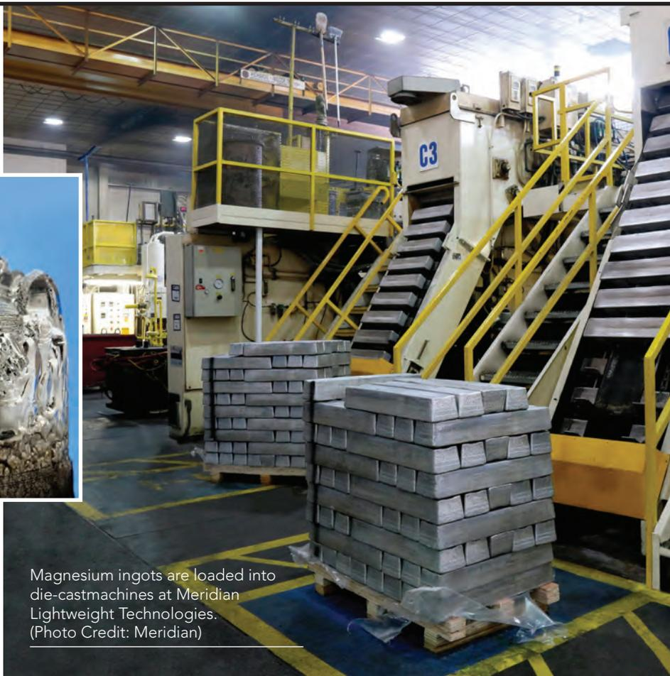
Magnesium ingots are loaded into die-cast machines at Meridian Lightweight Technologies. (Photo Credit: Meridian)
